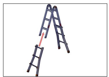
10. Re-insert the outer assembly onto the inner assembly. Make sure all components are secure and working properly before returning ladder to service.
