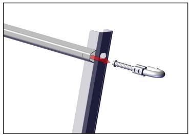
5. Pull the lock tab free of the rung, and discard.
